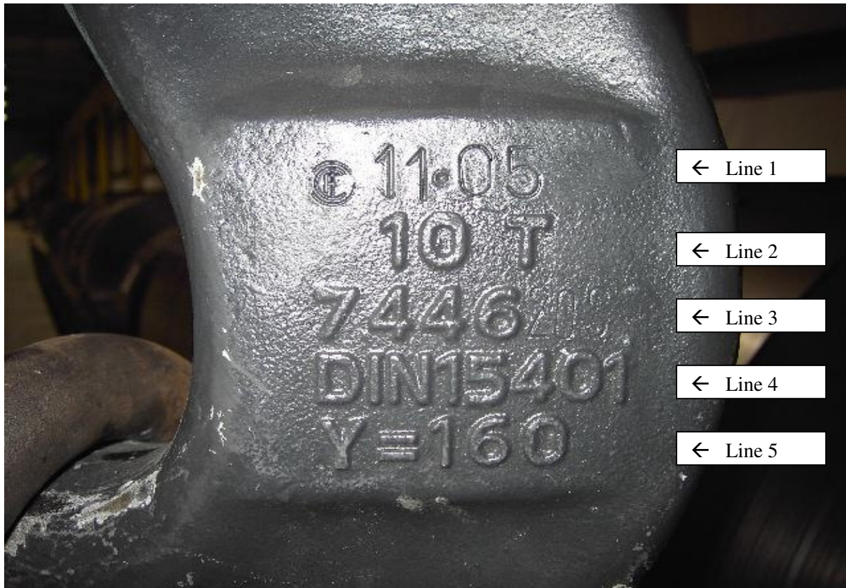
An example of markings on an RSN10 size load hook.
