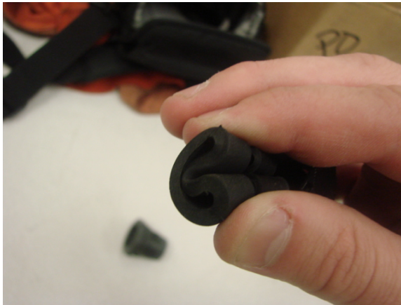
Fold round end of rubber boot
