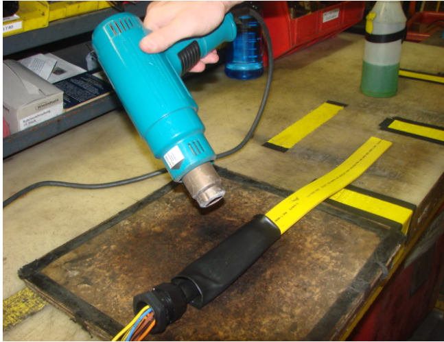
Applying heat to shrink tube
