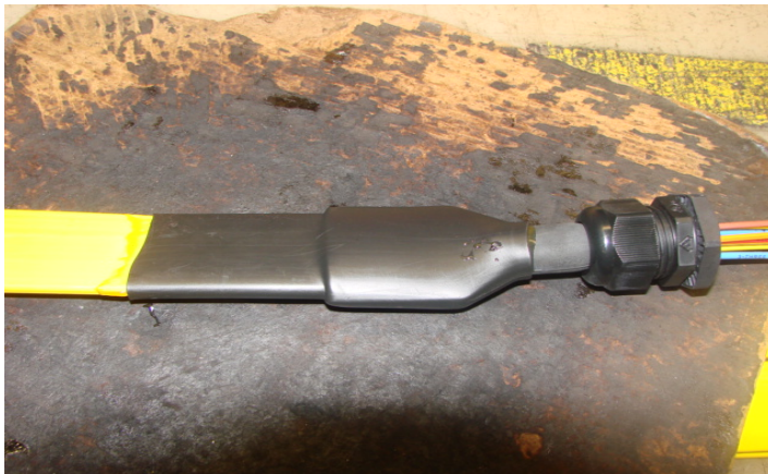
Completed flat cable adaptation
