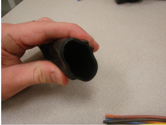
Squeeze flat end of boot to form a round opening
