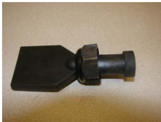
Flat cable boot with nut installed
